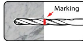
1. Drilling hole with recommended diameter and depth.
